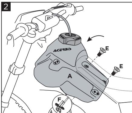
**Mount the original tap (F) on the Acerbis tank (A) and place it on the motorcycle. Insert the original screws (E) as shown in the figure.**
