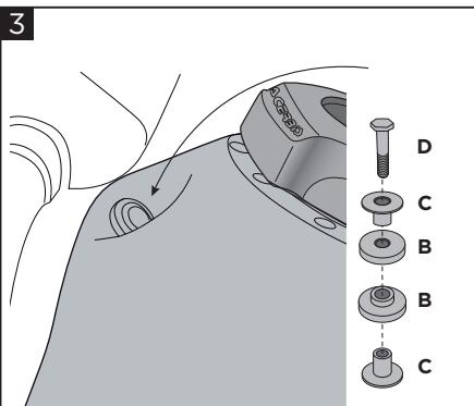
**Insert the screw (D), the bushings (C) and bushings (B) onto the front part of the tank.**
