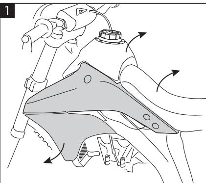
**Remove the saddle and side panels e remove the original tank.**
